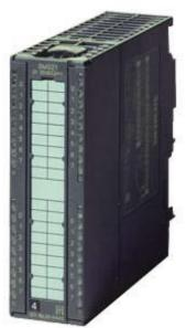
SIMATIC S7/PCS7 Digital input SM 321, 16 DI; 24 V DC, 1 x 40-pole, diagnostics-capable, for contacts (wired/ not wired), NAMUR encoder, 3/4-wire Bero, with chatter monitoring; Pulse extension, open-circuit detection Interface module IM 153-2 HF or IM 153-4 HF possible
