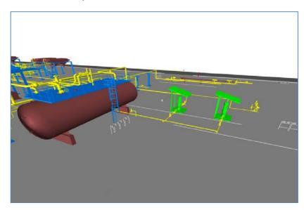
**6.3** Shelter of Chemical Injection Packages should be rotated 90 degree and access room to be provided by moving Slug Drums to East.
