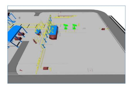
**6.10** After receiving vendor data, Piping route of Inlet Lines of Gas Compressors for avoiding any pocket to be reviewed and if required to be modified.
