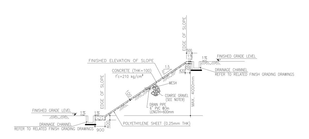
CONCRETE SLOPE PROTECTION WITHOUT BERM
