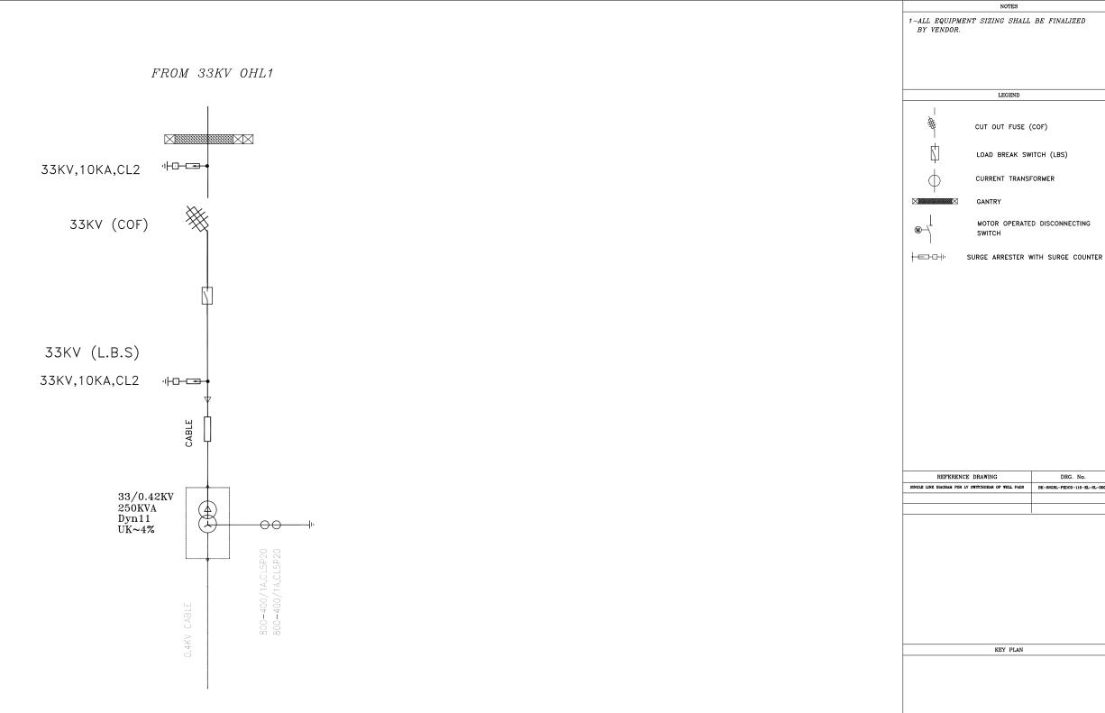
EQUIPMENT FOR OUTDOOR SUBSTATION IN WELL No BK14
