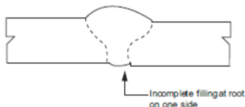
Figure 14—Inadequate Penetration Due to High-low
