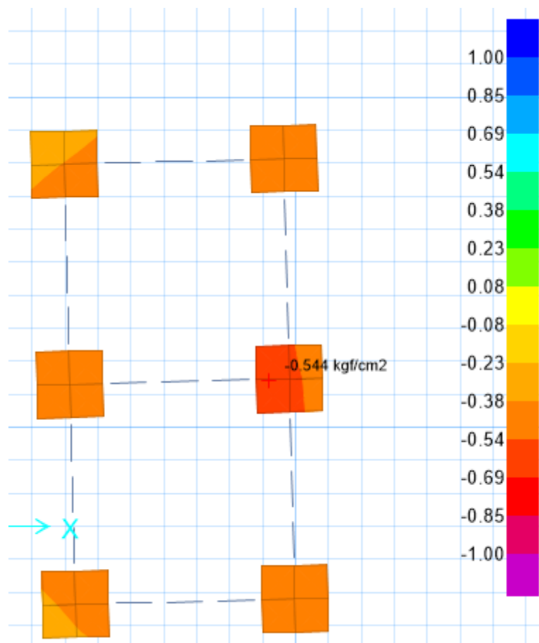
FIGURE 22 - Check of Stress for Foundation (kg/cm 2 )
