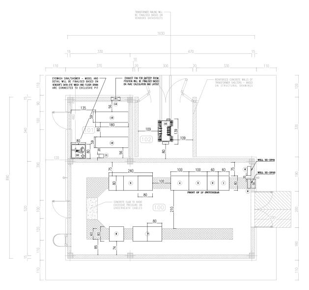
FLOOR PLAN OF WELL PAD SWITCHGEAR
