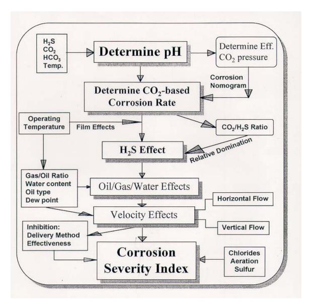
The first step in corrosivity determination is computation of the system pH, since it is the hydrogen ion concentration that drives the anodic dissolution. For production environments, where it is the dissolved CO<sub>2</sub> or H<sub>2</sub>S that contribute significantly to a suppressed pH, the pH can be determined as
