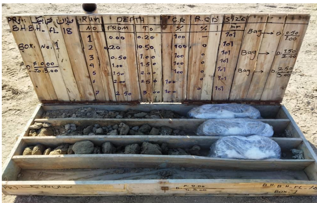
FL-18-CoreBox 1-Depth (0.0-3.0 m)
