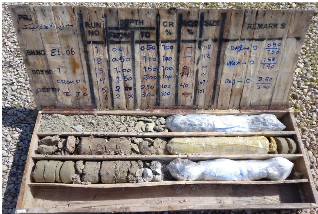
EL-06-CoreBox 1-Depth (0.0-3.0 m)
