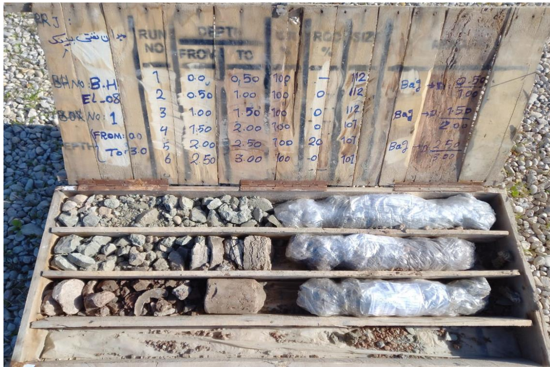
EL-08-CoreBox 1-Depth (0.0-3.0 m)
