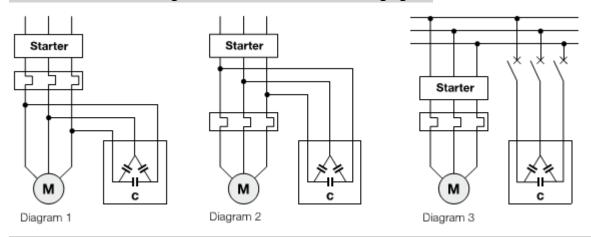
In the case of direct connection (diagrams 1 & 2), there is a risk of that after disconnection of the supply, the motor will continue to rotate (residual kinetic energy) & self-excite with the reactive energy supplied by the capacitor bank, acting as an asynchronous generator. In this case, the voltage is maintained on the load side of switching & control device, with the risk of dangerous overvoltage of up to twice the rated voltage value. Therefore total capacity should not be more
