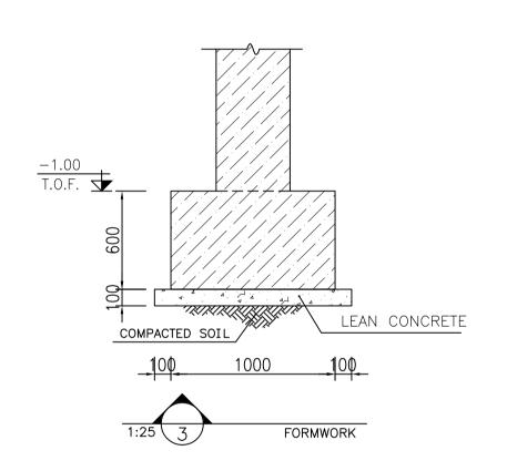
FOUNDATION FORMWORK PLAN
