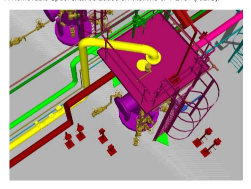
**6.7** All instrument branch of gas cooler outlet line shall be moved to near of related platform.
