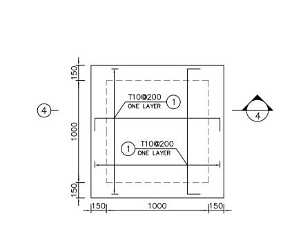
FOUNDATION REINFORCEMENT PLAN
