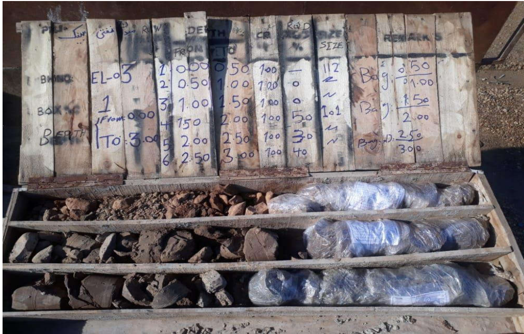
EL-03-CoreBox 1-Depth (0.0-3.0 m)
