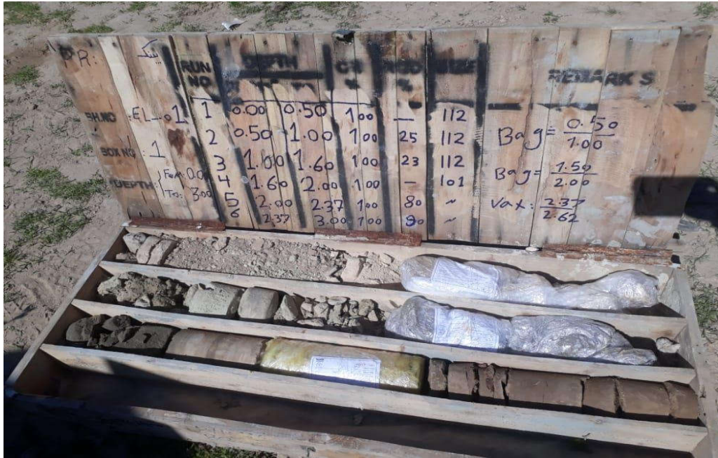
EL-01-CoreBox 1-Depth (0.0-3.0 m)
