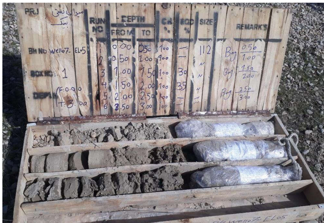
EL-05-CoreBox 1-Depth (0.0-3.0 m)
