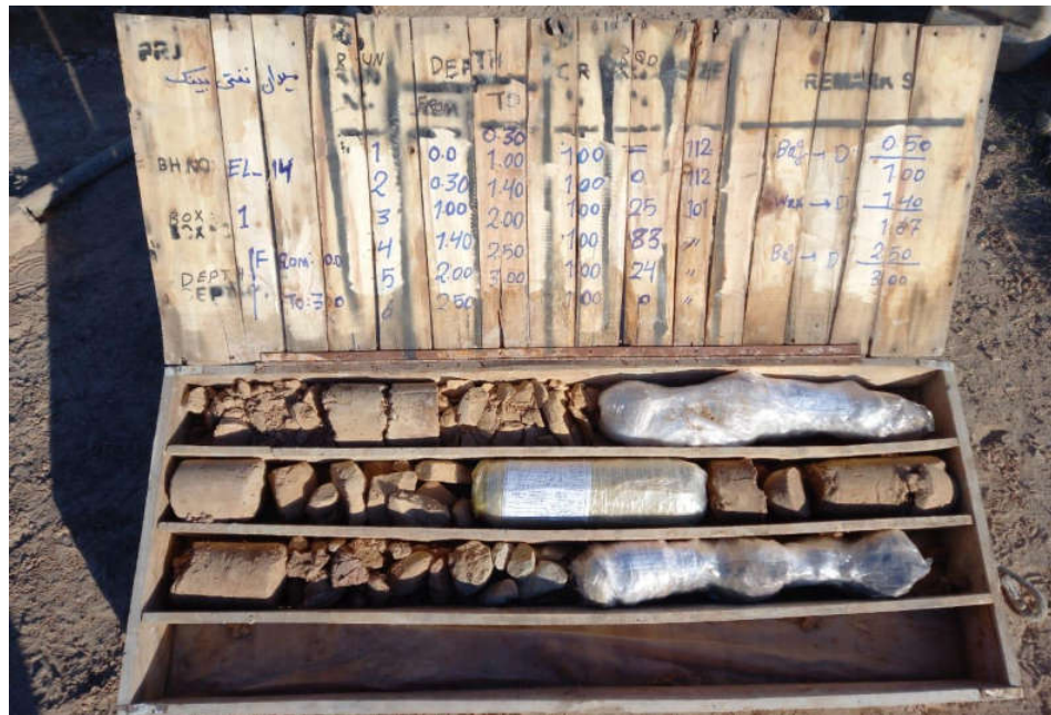
EL-14-CoreBox 1-Depth (0.0-4.0 m)
