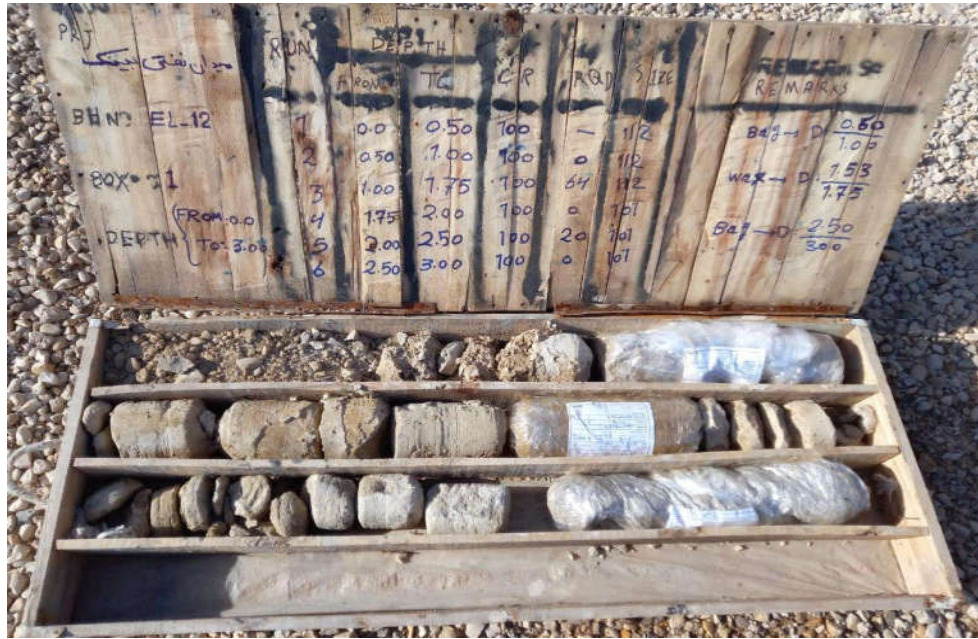
EL-12-CoreBox 1-Depth (0.0-4.0 m)
