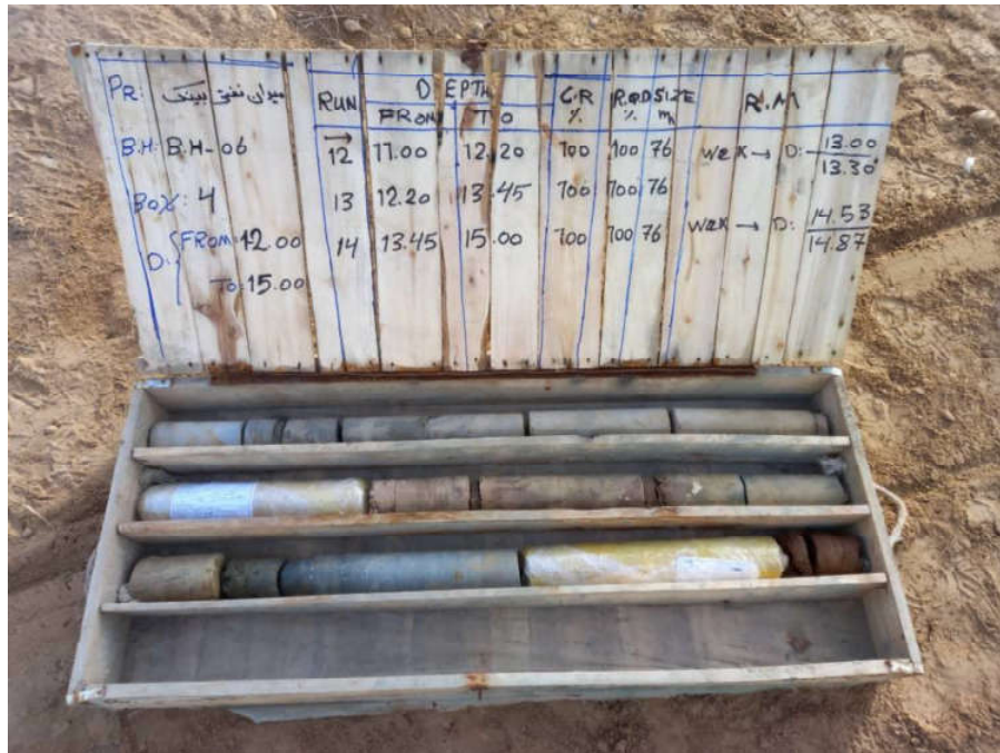
BH-06-CoreBox 4-Depth (12.0-15.0 m)
