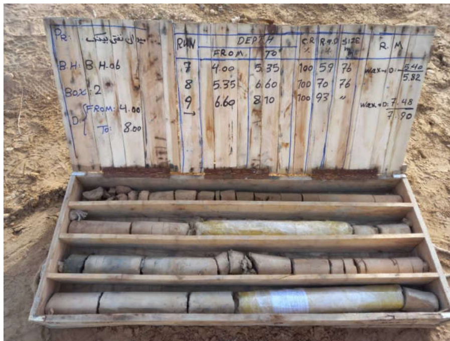
BH-06-CoreBox 2-Depth (4.0-8.0 m)
