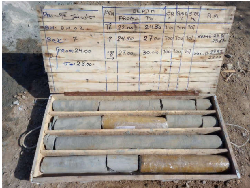
BH-02-CoreBox 7-Depth (24.0-28.0 m)
