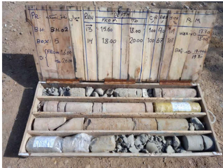
BH-02-CoreBox 5-Depth (16.0-20.0 m)
