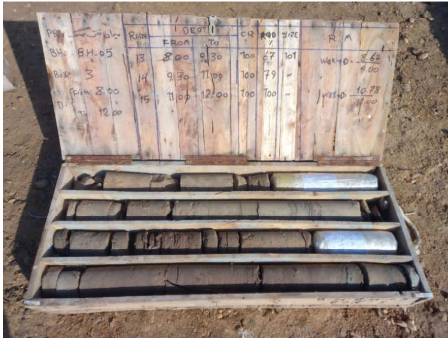
BH-05-CoreBox 3-Depth (8.0-12.0 m)
