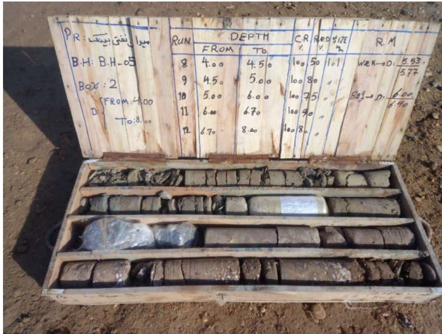
BH-05-CoreBox 2-Depth (4.0-8.0 m)
