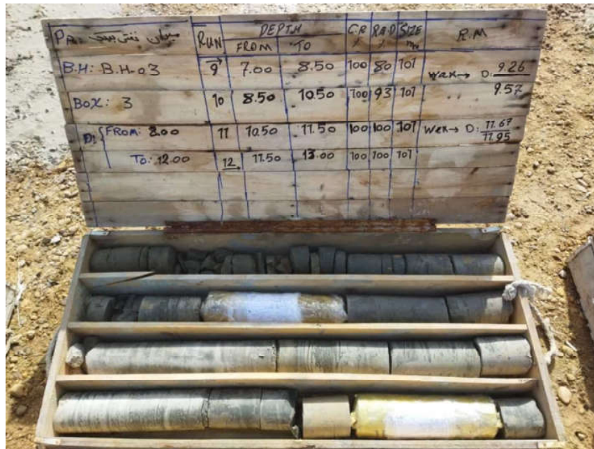
BH-03-CoreBox 3-Depth (8.0-12.0 m)
