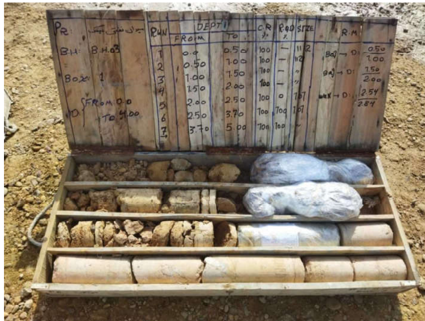
BH-03-CoreBox 1-Depth (0.0-4.0 m)
