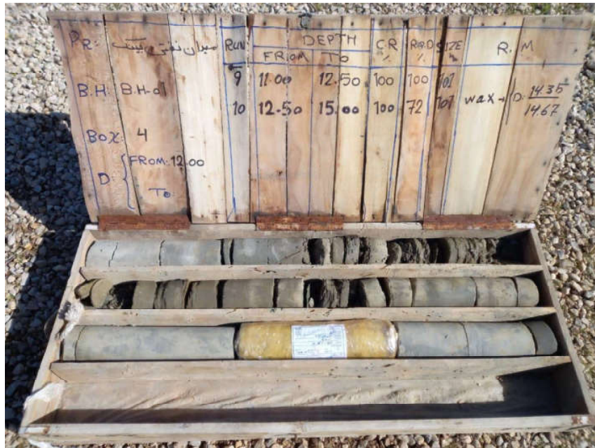
BH-01-CoreBox 4-Depth (12.0-15.0 m)
