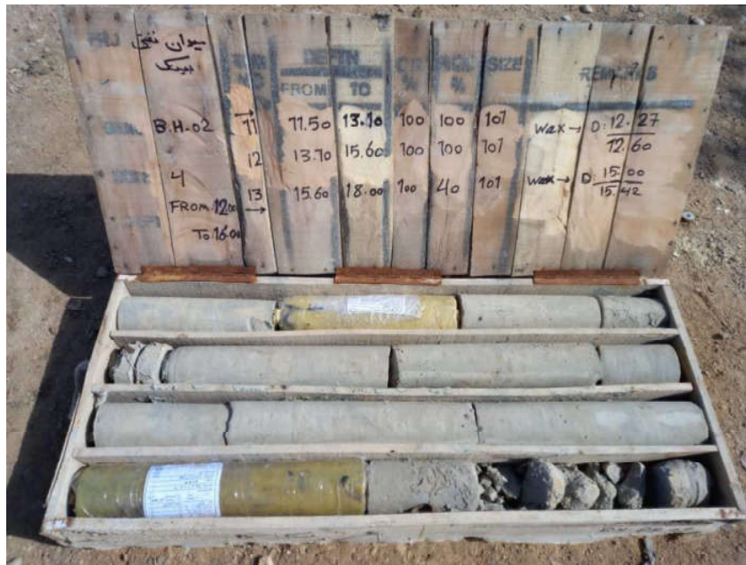
BH-02-CoreBox 4-Depth (12.0-16.0 m)
