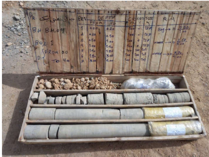
BH-04-CoreBox 1-Depth (0.0-4.0 m)
