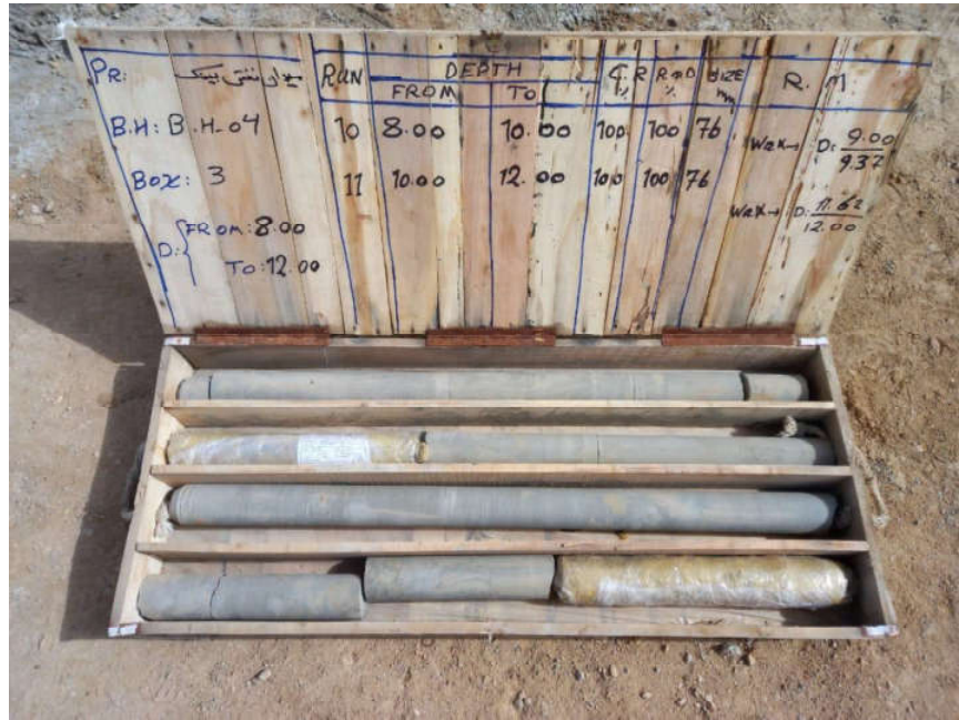
BH-04-CoreBox 3-Depth (8.0-12.0 m)
