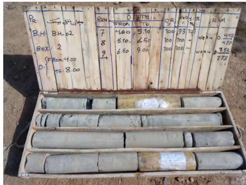
BH-02-CoreBox 2-Depth (4.0-8.0 m)
