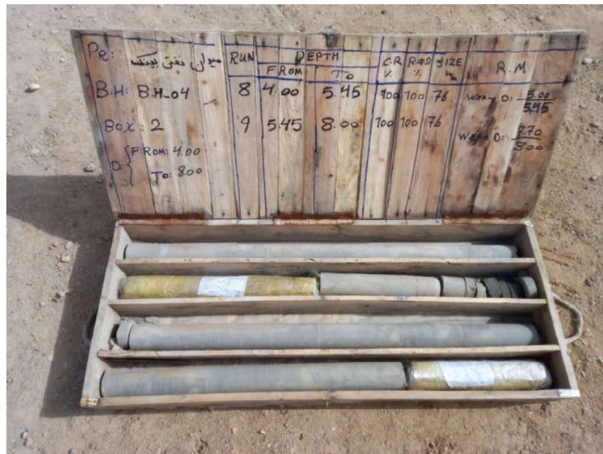
BH-04-CoreBox 2-Depth (4.0-8.0 m)
