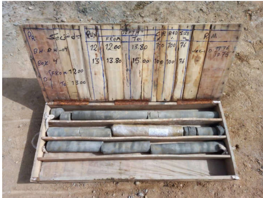
BH-04-CoreBox 4-Depth (12.0-15.0 m)
