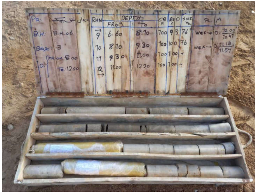
BH-06-CoreBox 3-Depth (8.0-12.0 m)
