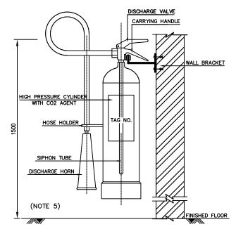
WALL MOUNTED PORTABLE CO2 EXTINGUISHER 4 SIDE VIEW
