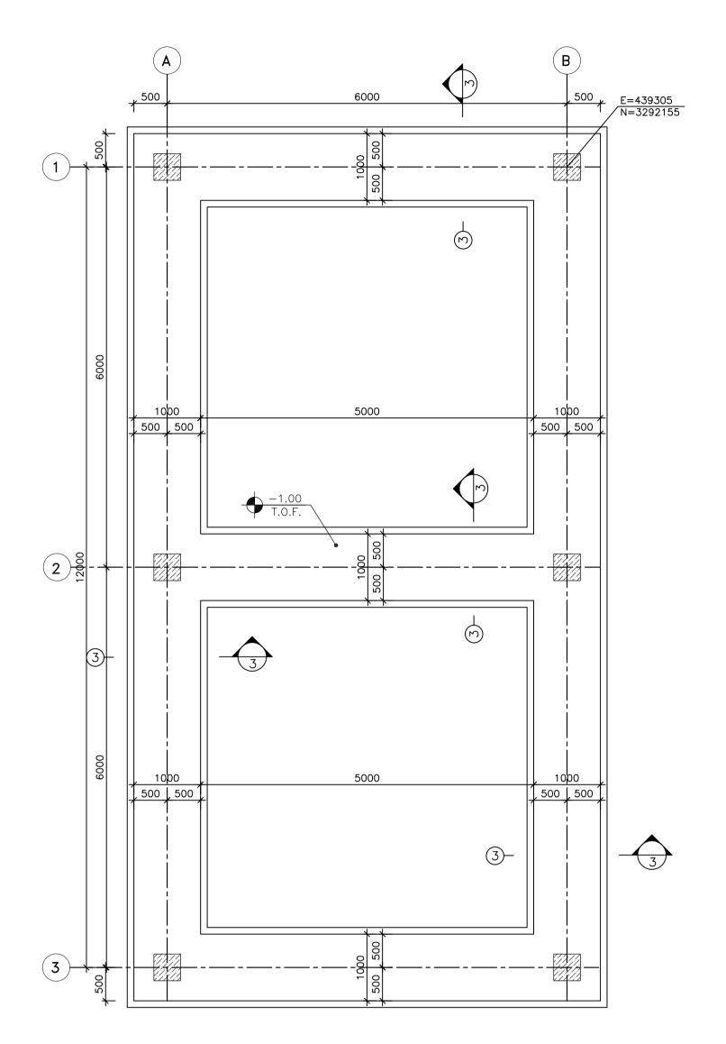
FOUNDATION FORMWORK PLAN
