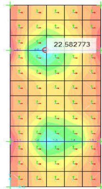
FIG 46 - max load combination on slab (M11=23.00 ton.m)
