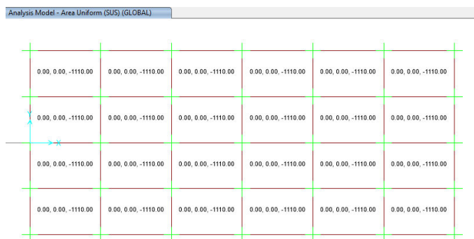
FIG 9 - applied soil load on foundation type A(1110Kg)
