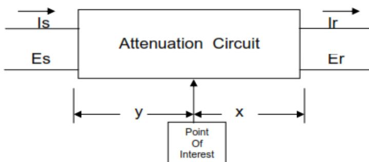
$$\alpha = \sqrt{rg} \quad \text{propagation or attenuation constant}$$
