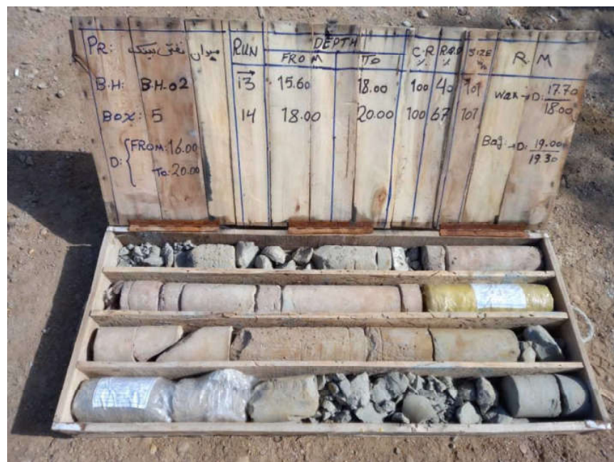
BH-02-CoreBox 5-Depth (16.0-20.0 m)
