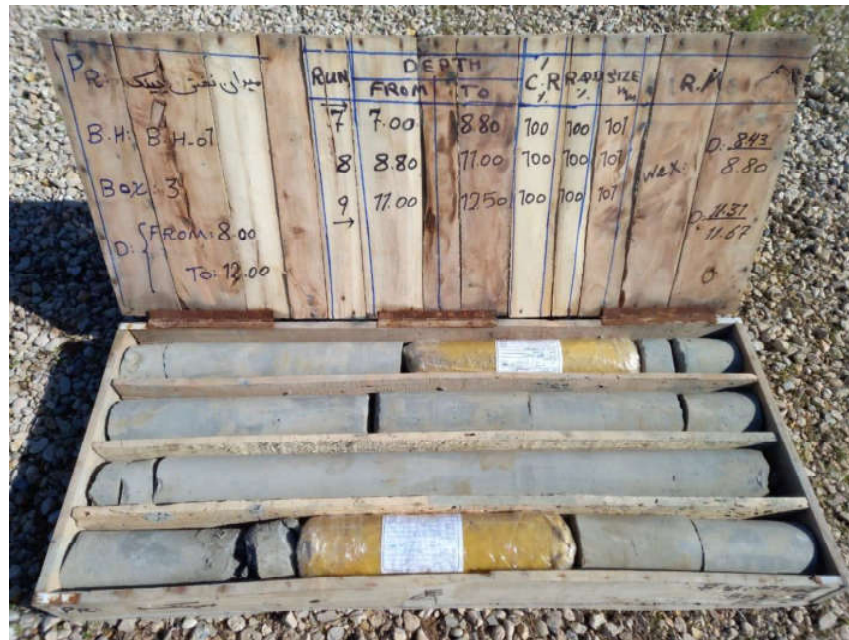
BH-01-CoreBox 3-Depth (8.0-12.0 m)
