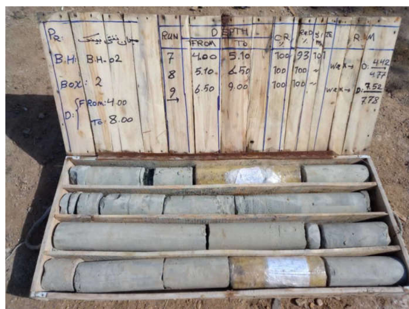
BH-02-CoreBox 2-Depth (4.0-8.0 m)
