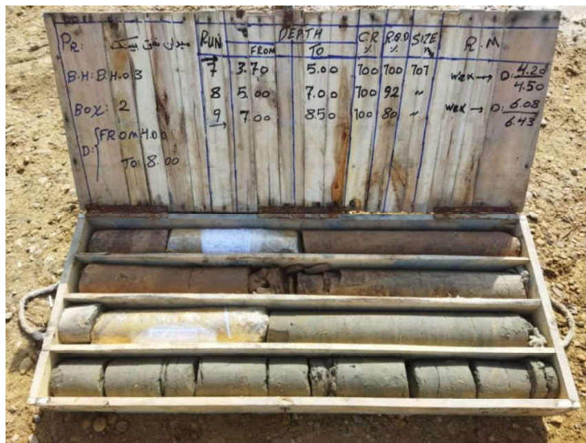
BH-03-CoreBox 2-Depth (4.0-8.0 m)
