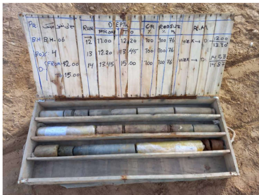
BH-06-CoreBox 4-Depth (12.0-15.0 m)
