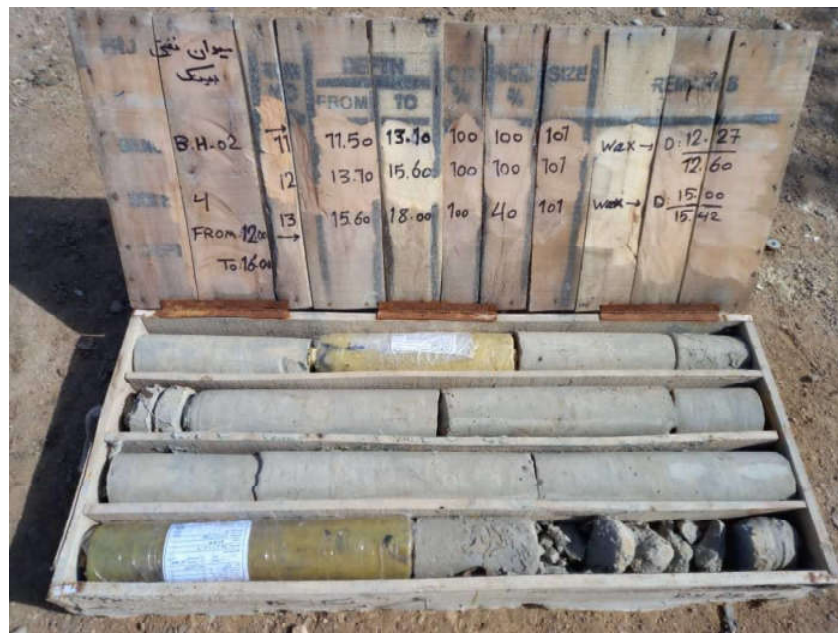
BH-02-CoreBox 4-Depth (12.0-16.0 m)
