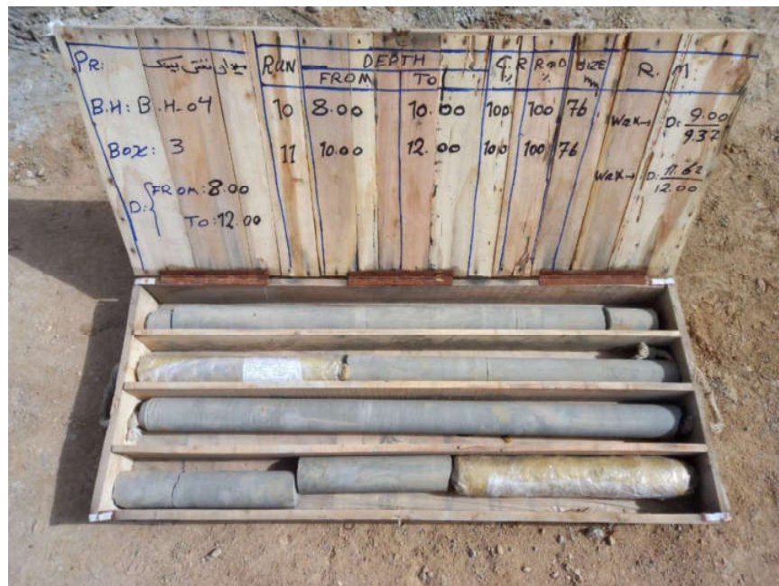
BH-04-CoreBox 3-Depth (8.0-12.0 m)
