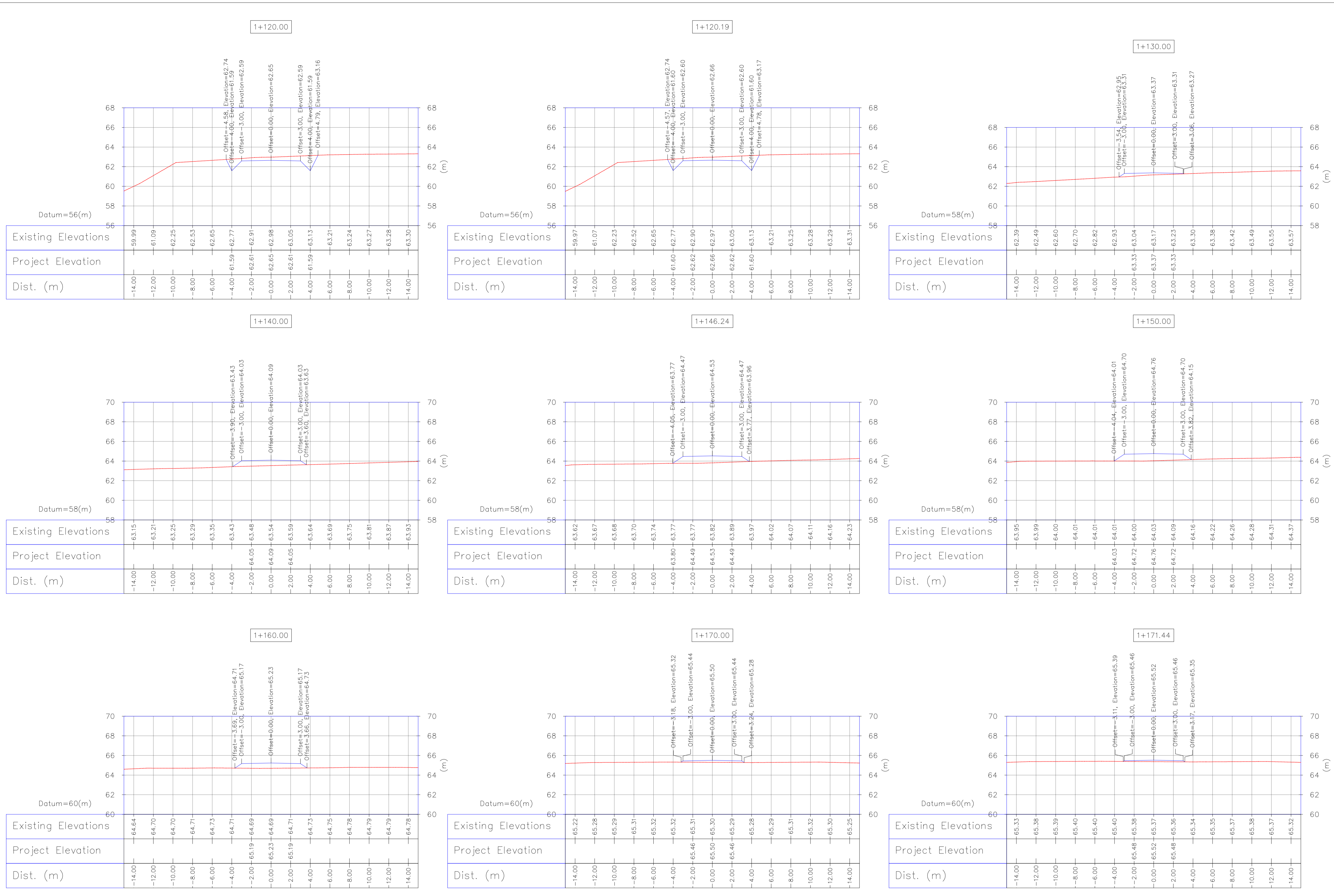
1:200 Wellpad Access Road Transversal Sections
