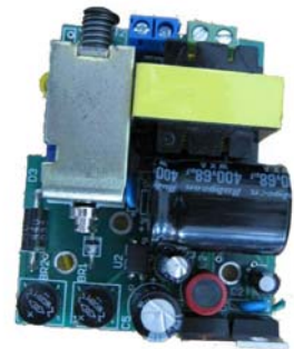
Remote reset circuit PT500-20
