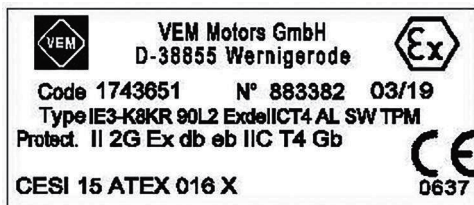
Nameplate for Ex d(e) motors with CESI certificate
