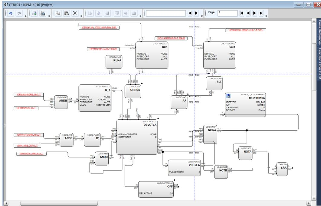
Figure Typical P1 (Single Motor With ESD Interlock)
