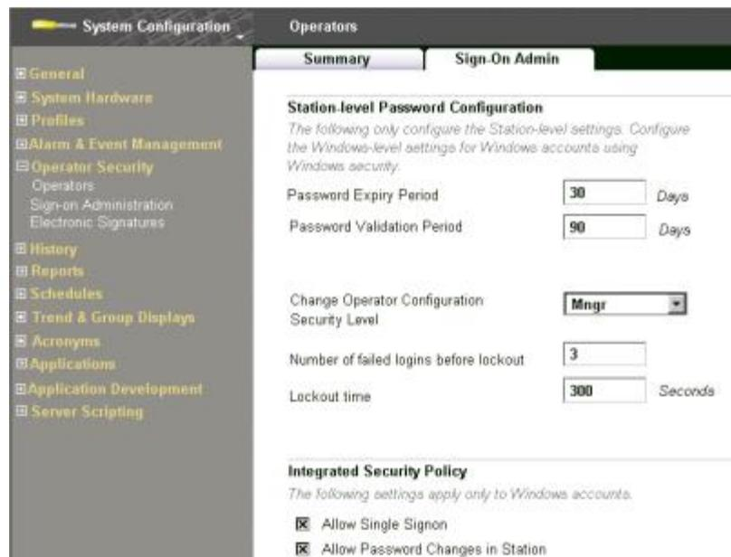
2. Click the Enable Single Sign On check box. Check mark appears in the check box, single sign on function is enabled, and only the Server Name field is accessible. Login is based on current Windows user account login to the named Server and the login dialog does not appear for subsequent logins.
