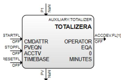
You specify a target value for the accumulator, and up to four trip points, which are "near" and "nearer to" the target value. The TOTALIZER block sets status flags to indicate when the accumulator value is near (and nearer to) the user-specified target values.
