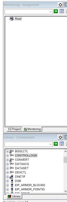
3. Click the appropriate tab (Project, Monitoring or Library) on the bottom of the tree window to select the desired tree view. Selected tree is displayed.
