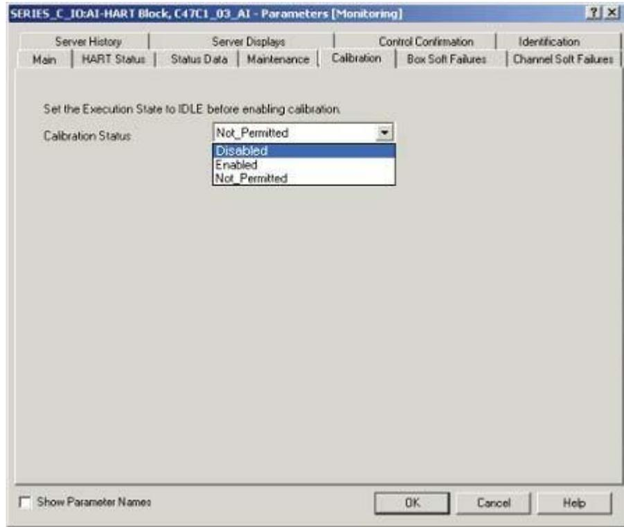
**Figure 37: Calibration tab**
