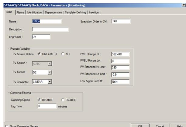
In this case range is between 0 to 382.448 , so the output will be 191.224 as see in below picture.
