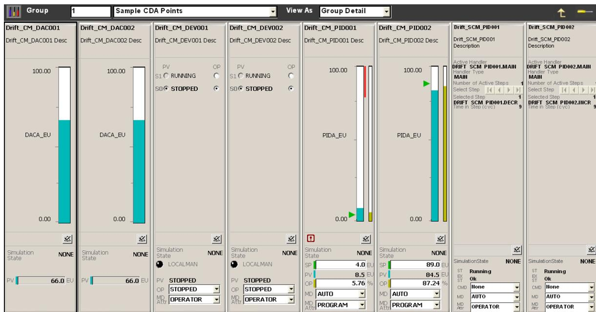
You can create custom Group Faceplate Template displays using Display Builder and then specify the template for particular points when you build the point.
