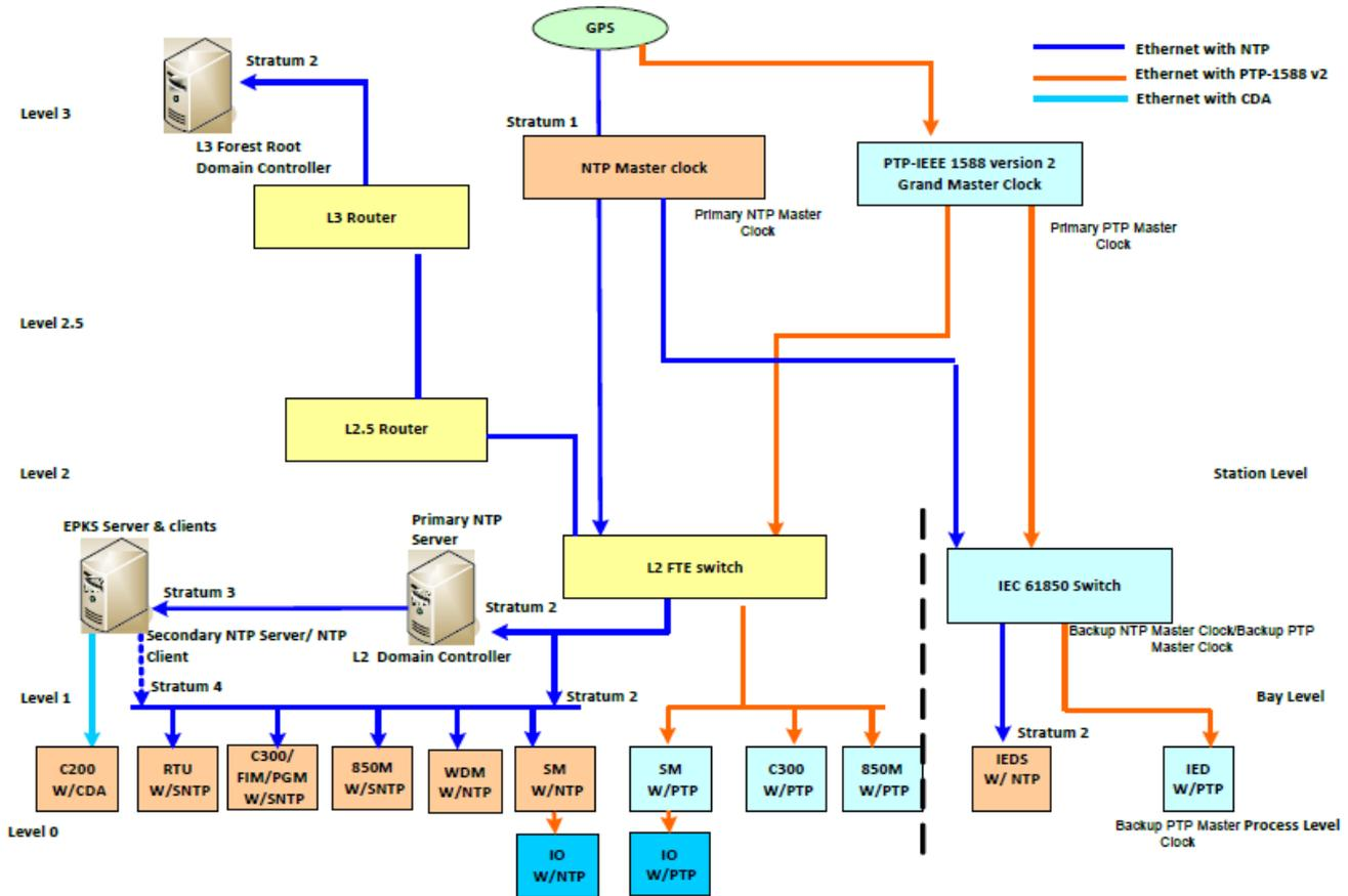
Typical time distribution topology that is supported by Experion connected devices.
