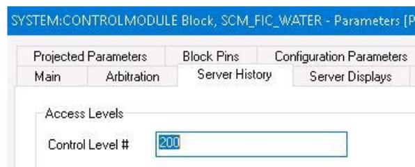
In Chart view or faceplate of the displayed point in station, if the Control level configured for this CM required is higher than the one defined for the logged user then the change is refused with a suitable system message
