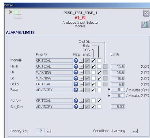
Detail Display for Alarms and Limits in Analog Input Family
