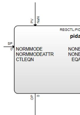
The PID block has two analog inputs - a process variable (PV) and a set point (SP). The difference between PV and SP is the error and this block calculates a control output (OP) that should drive the error to zero.
