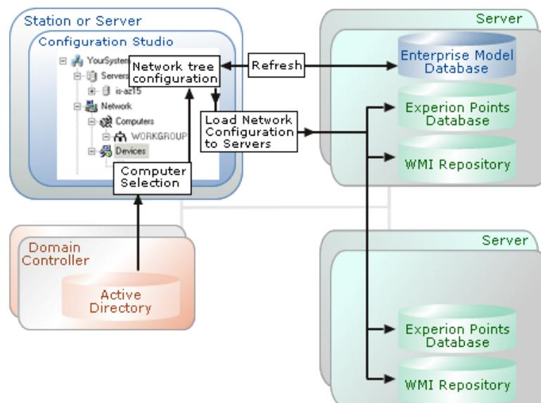
If there is an inconsistency of the Network tree configuration between the EMDB and the Experion database, icons appear in the Network tree in Configuration Studio.
