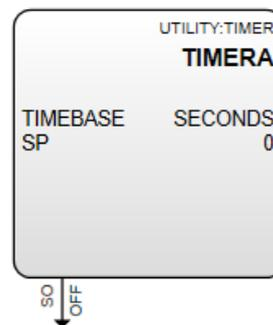
Used to keep track of elapsed time during a process and provides indication when elapsed time reaches predefined limit. The TIMEBASE can be configured to represent seconds, minutes, or cycles (number of execution cycles).
