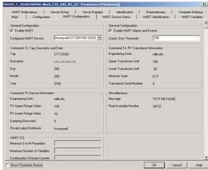
**Figure 43: HART Configuration tab**
