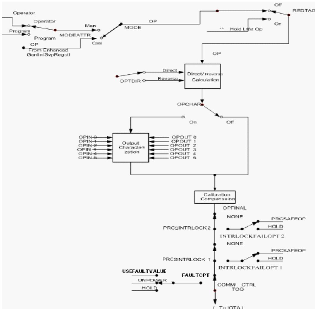
AO block execution diagram when OPACTION is “FullValue”
