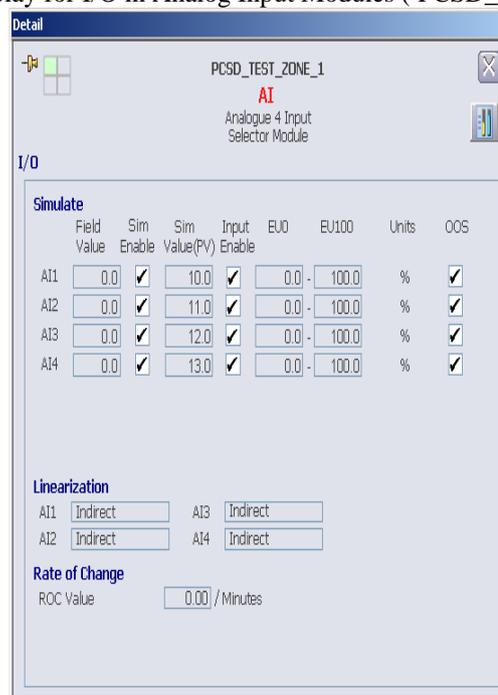
Detail Display for I/O in Analog Input Family except \_AI\_SCADA\_130, \_AI\_SLMG\_130 control modules
