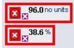
This dynamo provides numeric indication of process value or any custom parameter value along with its engineering unit.
