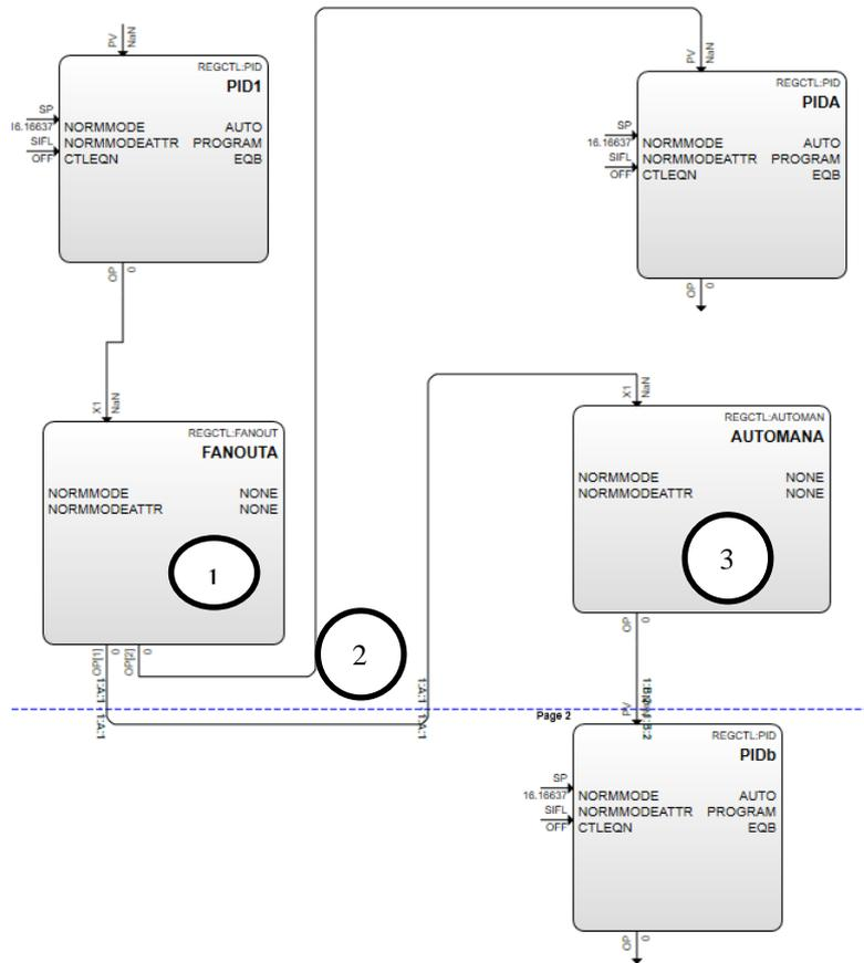
Example of CB configuration using AUTOMAN block
