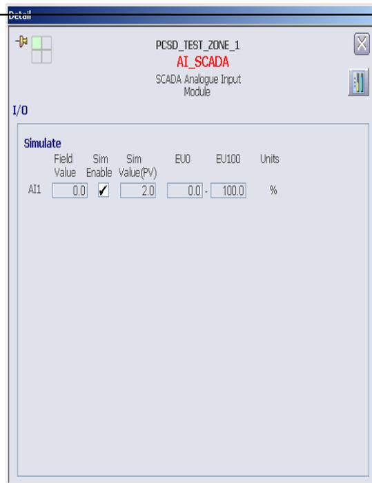
Detail Display for I/O in \_AI\_SCADA\_130 module
