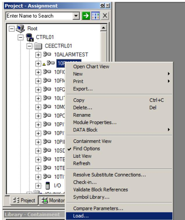
At the same time, make sure that the desired module is assigned to the desired HMI screen, otherwise the module control will not be correctly placed in the monitoring mode after downloading.
