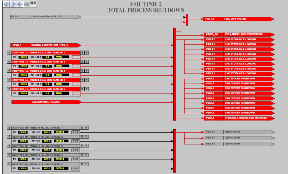
The dynamic elements on the Cause and Effect display will utilize the Emerson standard dynamos which are modified to suit need.
