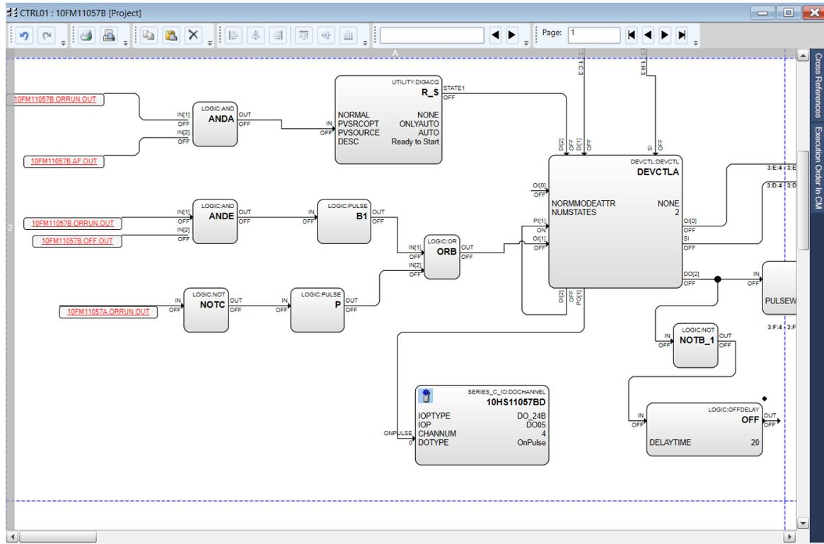
The only different between duty standby (PUMP,MOTOR,FAN,...) and the single one is in DEVCTL pin(OI[1]) that its linked to the other stand by device in case of that if the ON device going OFF , the standby device going ON.
