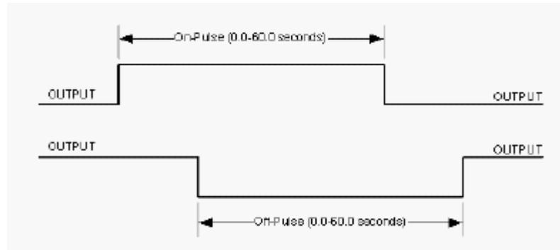
On-Pulse and Off-Pulse Output types
