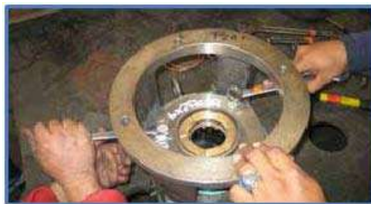
Figure 8.19 Tightening the bolts.
