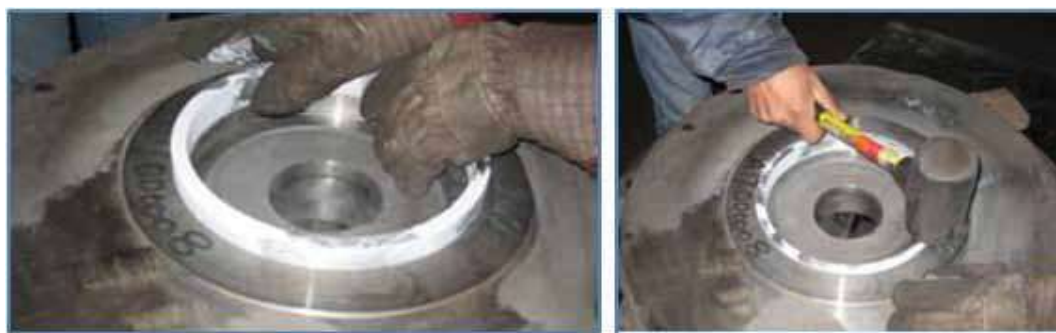
Figure 8.25 Positioning the wear ring.
