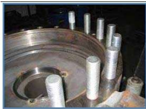
Figure 8.38 Positioning the studs manually.
