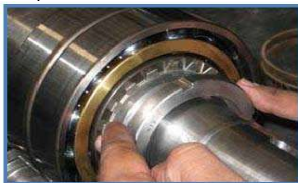
Figure 8.5 Positioning the locknut.
