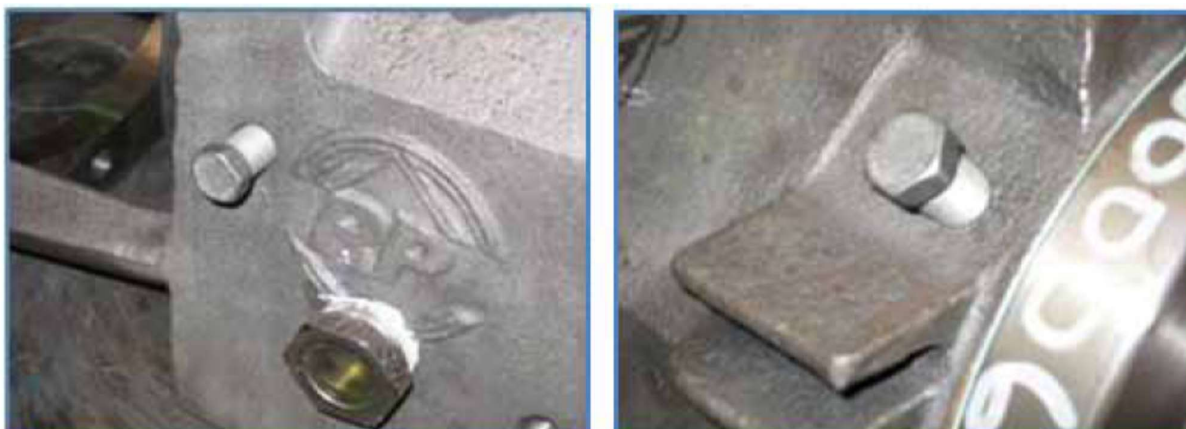
Figure 8.24 Identifying the plugs in the bearing bracket.
