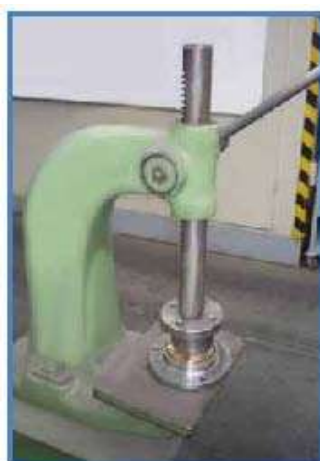
Figure 8.15 Inserting the labyrinth seal.
