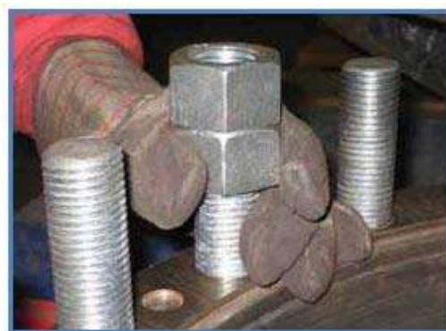
Figure 8.39 Tightening the studs.
