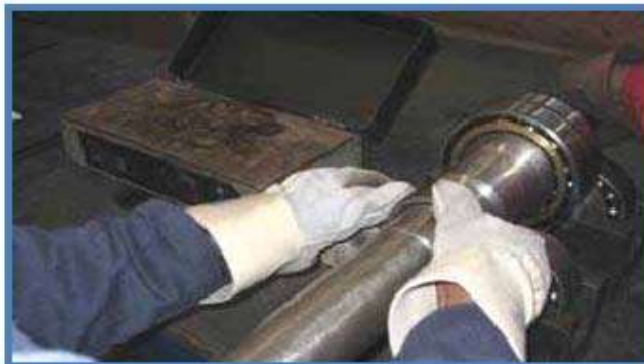
Figure 8.12 Positioning the radial roller bearing's inner race.
