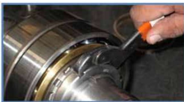
Figure 8.6 Tightening the locknut.
