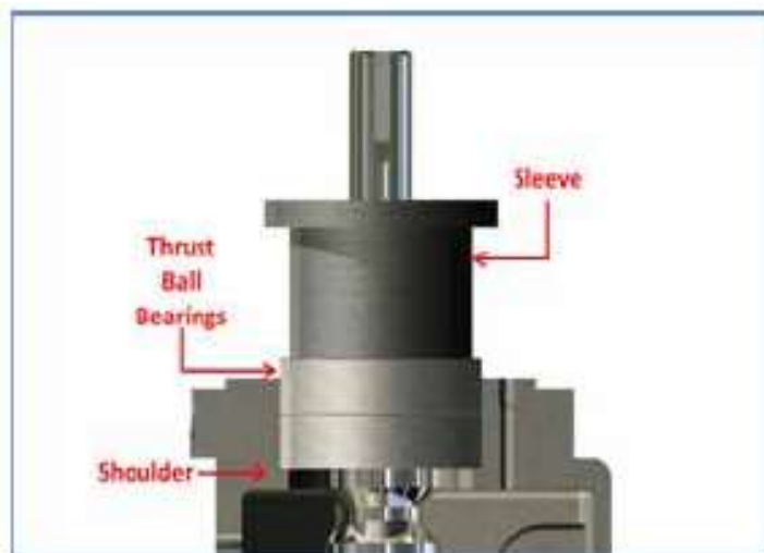
Figure 8.22 Ensuring bearings are in contact with the shoulder of the bearing housing.
