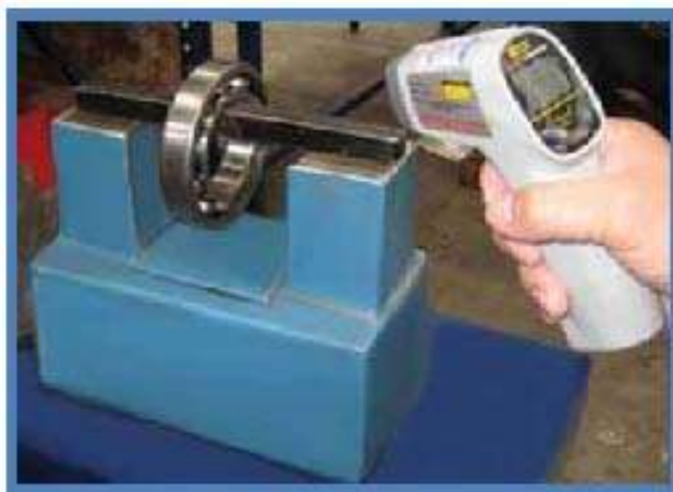
Figure 8.1 Heating the thrust bearings.
