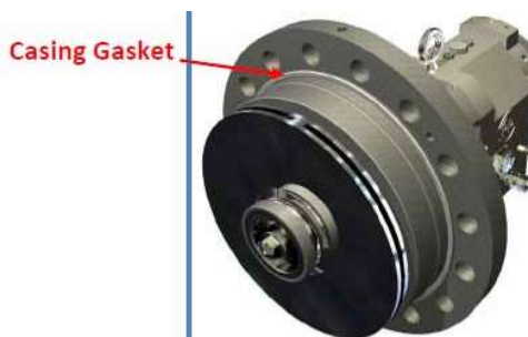
Figure 8.41 Identifying the casing gasket.
