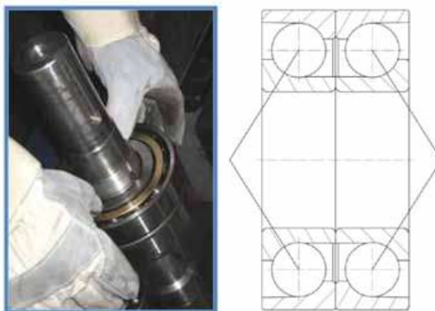
Figure 8.3 Positioning the thrust bearings.
