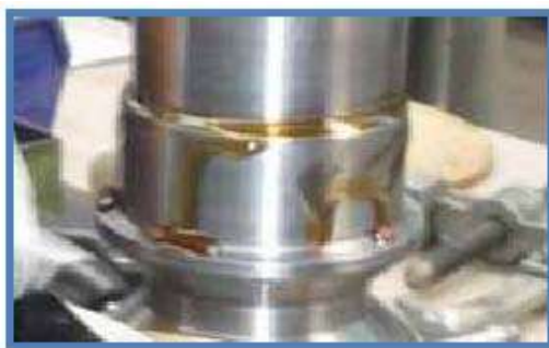
Figure 8.2 Lubricating the shaft.
