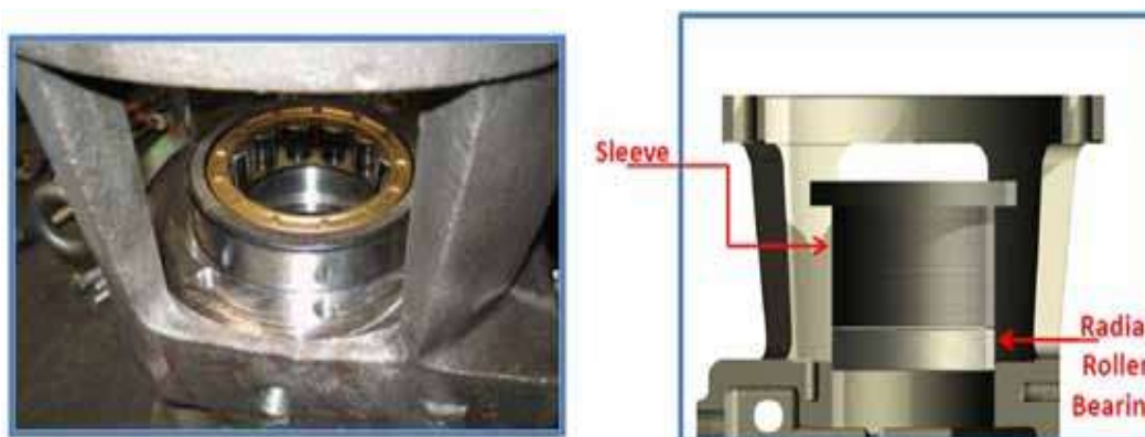
Figure 8.16 Inserting radial roller bearing.
