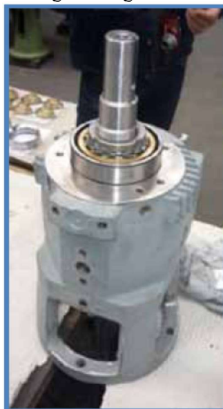
Figure 8.20 Positioning the rotor assembly on the bearing bracket.
