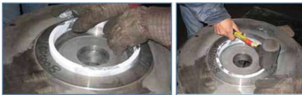
Figure 8.25 Positioning the wear ring.
