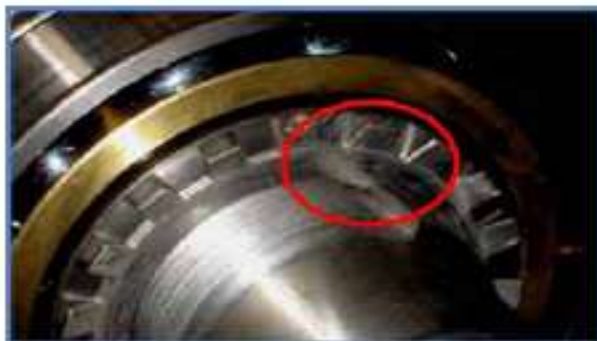
Figure 8.4 Positioning the lock washer.
