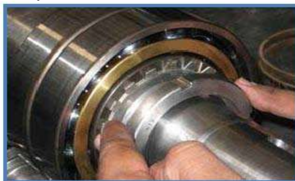
Figure 8.5 Positioning the locknut.
