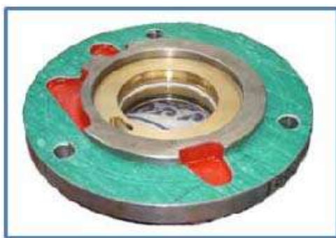
Figure 6.17 Positioning the radial gasket.
