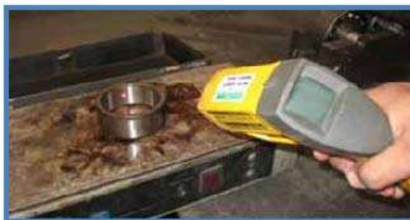
Figure 8.9 Heating the inner race of the radial roller bearing.
