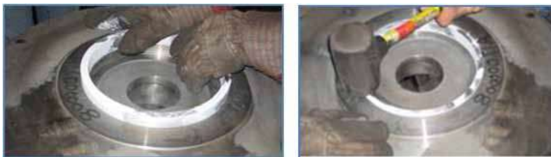
Figure 8.28 Positioning the wear ring.
