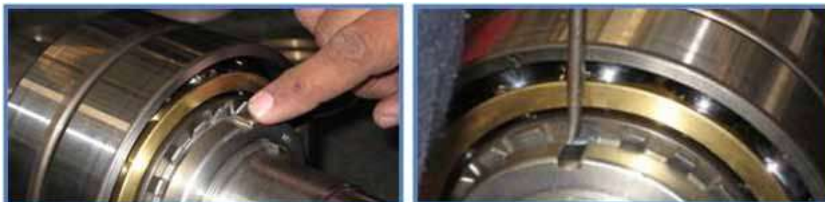
Figure 8.7 Bending a tab of the lock washer in the locknut.
