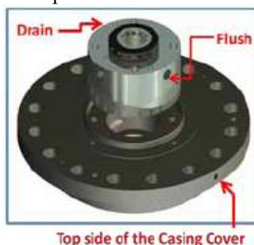
Figure 8.31 Verifying the drawing of the mechanical seal.
