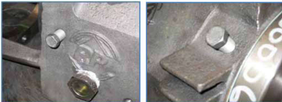
Figure 8.24 Identifying the plugs in the bearing bracket.
