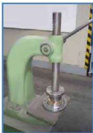
Figure 8.15 Inserting the labyrinth seal.
