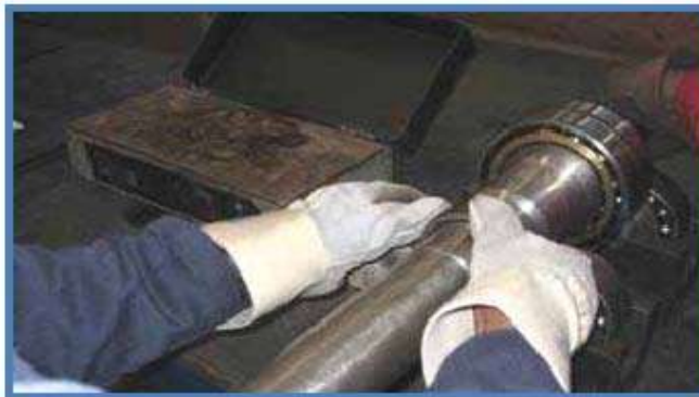
Figure 8.12 Positioning the radial roller bearing's inner race.
