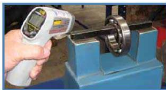
Figure 8.8 Heating the radial ball bearing.
