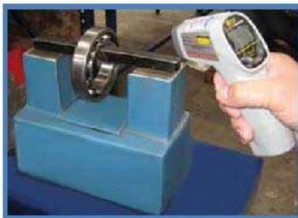
Figure 8.1 Heating the thrust bearings.
