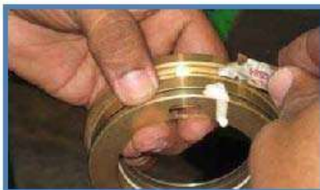
Figure 8.14 Lubricating the labyrinth seal.
