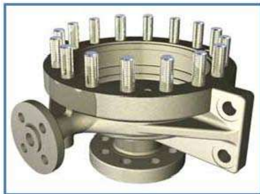
Figure 8.40 Visual inspection of the studs.
