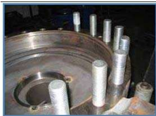
Figure 8.38 Positioning the studs manually.
