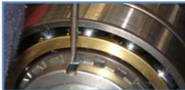
Figure 13.7 Bending a tab of the lock washer in the locknut.
