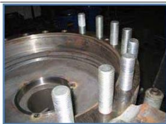
Figure 13.38 Positioning the studs manually.
