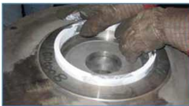
Figure 13.25 Positioning the wear ring.
