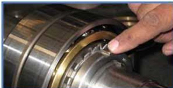
Figure 13.7 Bending a tab of the lock washer in the locknut.
