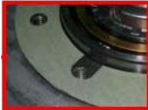
Figure 13.23 Positioning the thrust gasket in the bearing housing.
