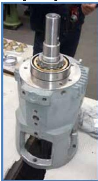
Figure 13.20 Positioning the rotor assembly on the bearing bracket.
