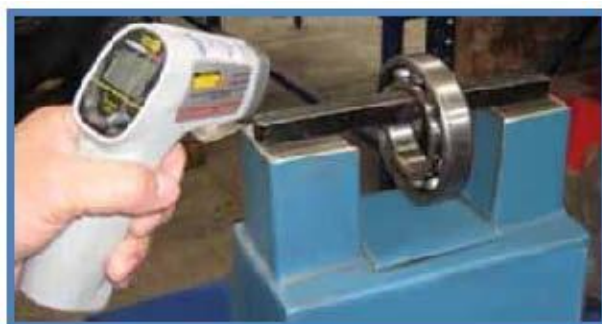
Figure 13.8 Heating the radial ball bearing.
