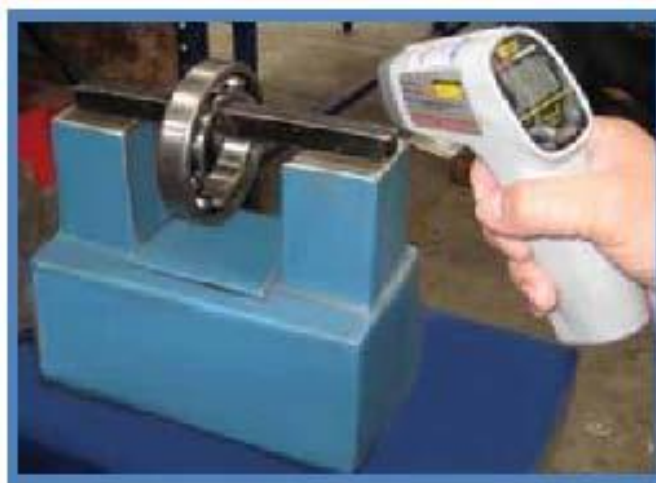
Figure 13.1 Heating the thrust bearings.
