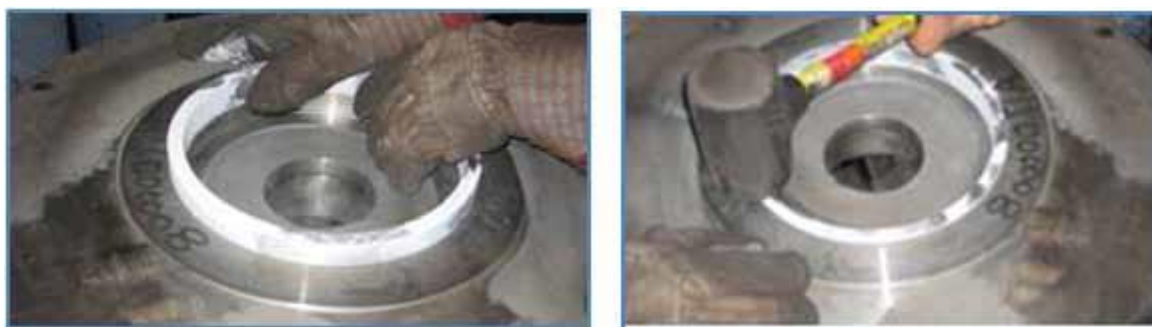
Figure 13.28 Positioning the wear ring.
