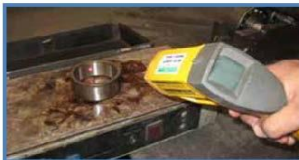
Figure 13.9 Heating the inner race of the radial roller bearing.
