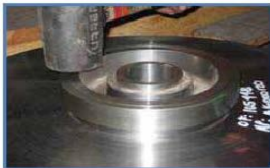
Figure 13.30 Positioning the wear rings of the impeller.
