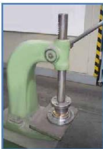
Figure 13.15 Inserting the labyrinth seal.
