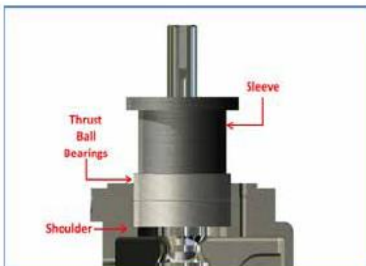
Figure 13.22 Ensuring bearings are in contact with the shoulder of the bearing housing.
