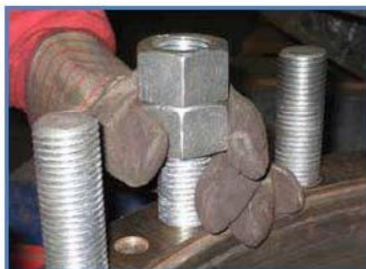
Figure 13.39 Tightening the studs.
