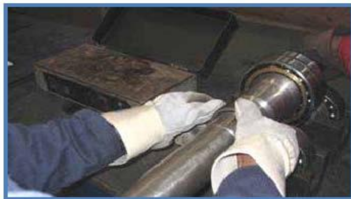
Figure 13.12 Positioning the radial roller bearing's inner race.
