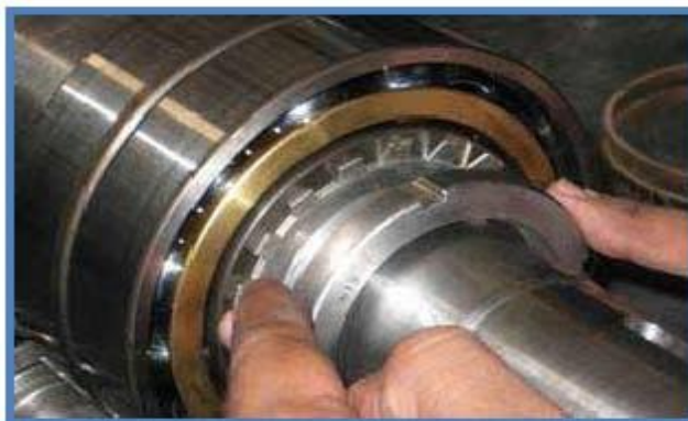
Figure 13.5 Positioning the locknut.
