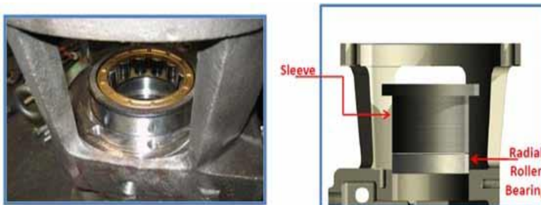
Figure 13.16 Inserting radial roller bearing.
