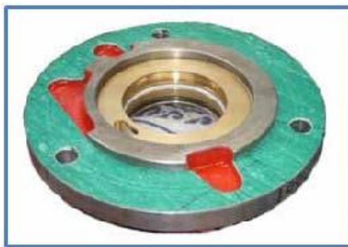
Figure 13.17 Positioning the radial gasket.
