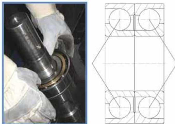
Figure 13.3 Positioning the thrust bearings.
