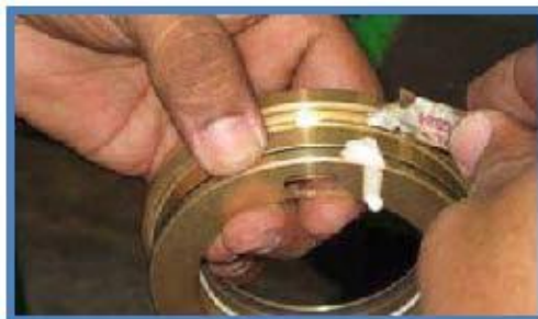
Figure 13.14 Lubricating the labyrinth seal.
